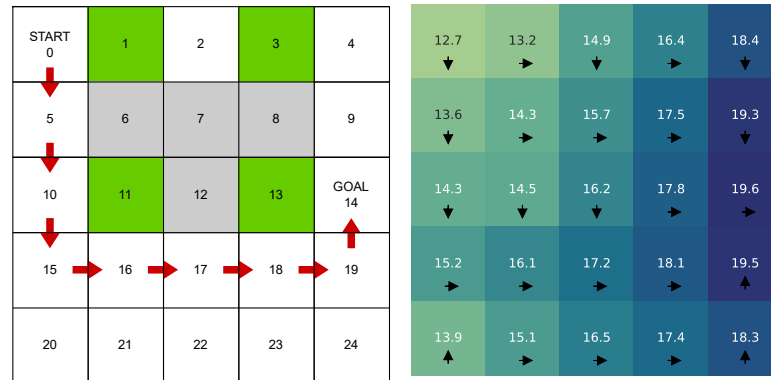
Figure 1. (Left) Representation of the environment, adapted from the first figure of Lopes et al. [1]. The green (light) states have uncertain transitions, the grey (dark) states incur a negative reward. The red arrows indicate the optimal path to the goal state. (Right) Implementation of the environment in Python, with the state values and optimal policies computed by value iteration.
