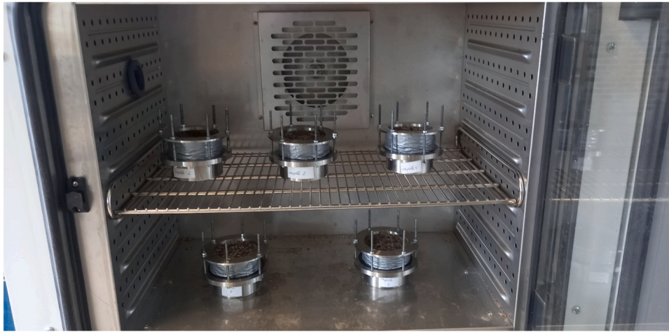
Fig. 2. S/BP samples having their sides sealed with waterproof aluminum tape and fixed at the top of cups enclosing a solution of potassium nitrate (KNO 3 ) at their bottoms.
