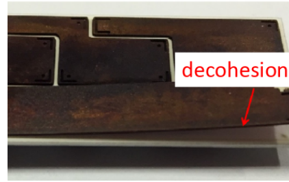
(b) ceramic-copper interface decohesion
