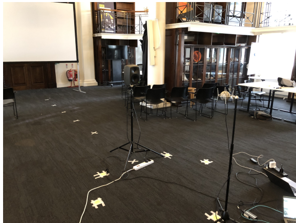
Fig. 1: SRIR measurement setup for the front position.
