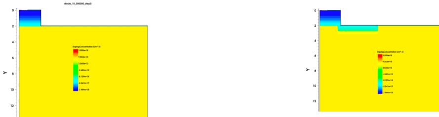
Fig. 3. Cross-section of the periphery protection (only half-cell to limit calculation time) of both diode structures with MESA (left) and MESA+JTE (right) defined with Sentaurus / Synopsys [4].
