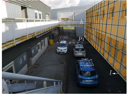
Fig. 6: The three experimental vehicles in an urban canyon. An example of a ND grid is represented on the right along with the facade plane and the normal vector in the middle l of the segment.
