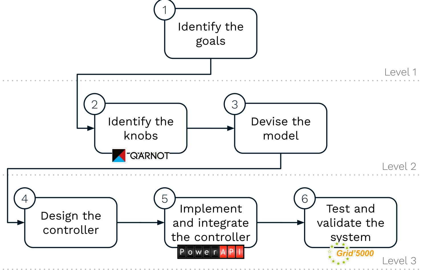
Step by step methodology to develop and validate a controller.
