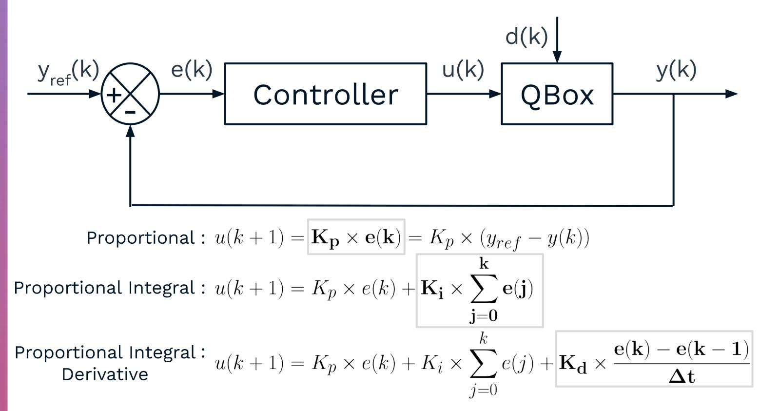
Control Theory consists in adapting dynamically the behavior of the selected system in order to reach the reference value. It requires instrumenting the infrastructure to implement sensors and actuators so that the controller can take decisions and interact with the system regarding the gap between the reference and the current state.
