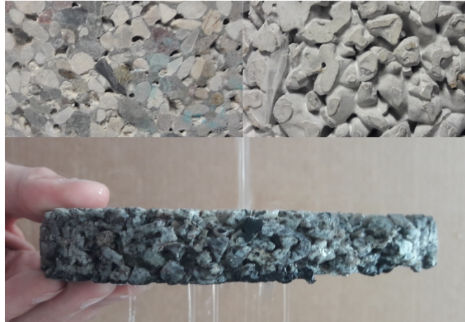
Figure 6: Examples of pervious concrete textures (top left and right) and demonstration of permeability (bottom)
