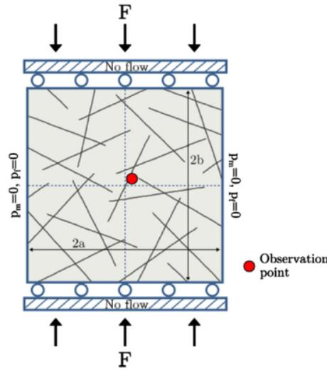
Figure 6: Problem used for benchmarking dual-continuum poroelastic models (Ashworth and Doster, 2019).
