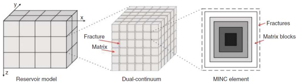
Figure 11: Concept of the multiple interacting continua (MINC) method ((Jiang et al., 2016) redesigned form of original (Pruess and Narasimhan, 1982).
