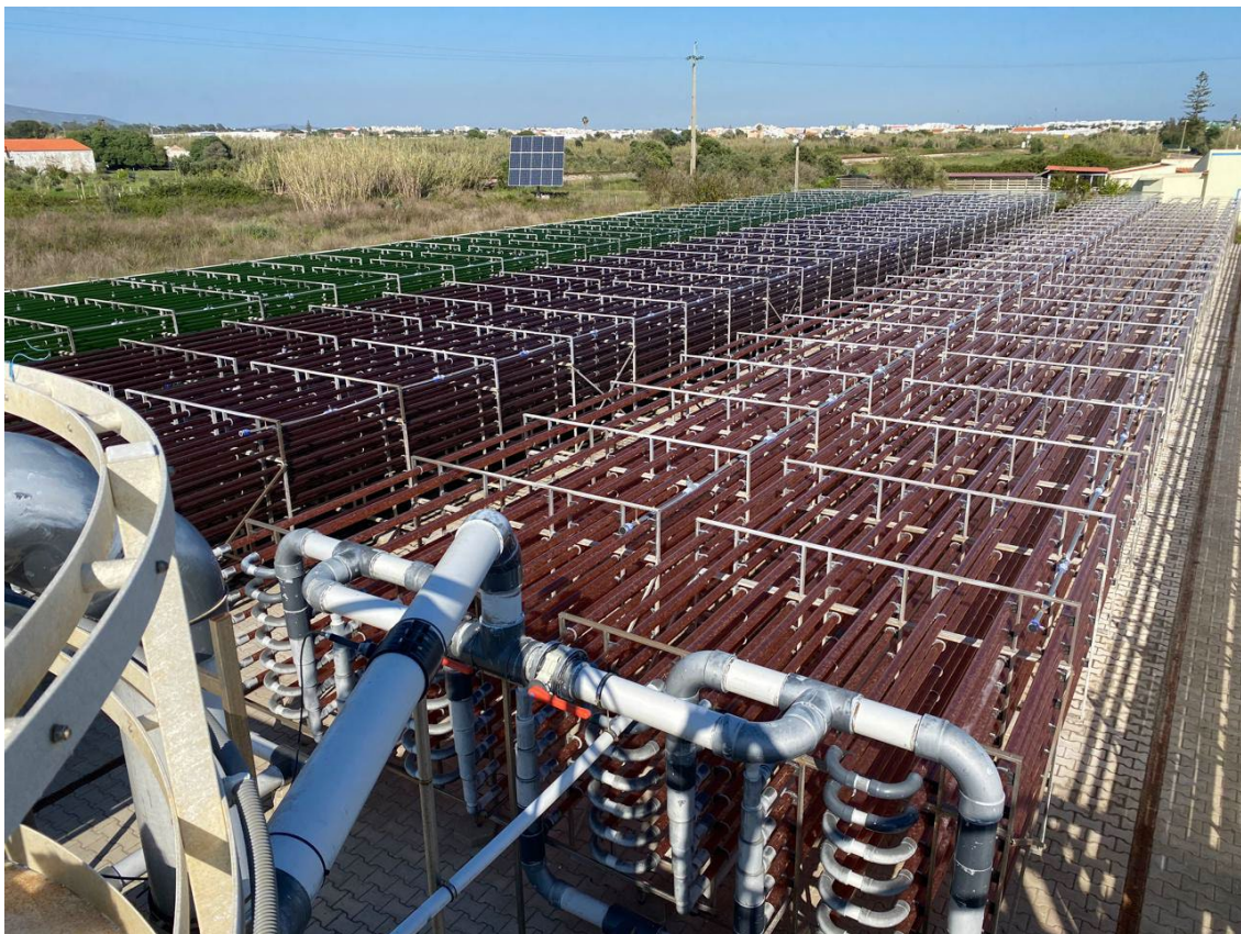
Figure 2.11 Production of microalgae in photobioreactors by Necton in the South of Portugal (Necton).
