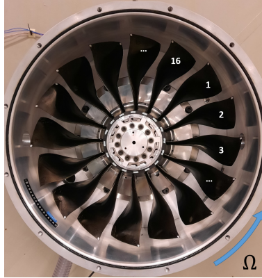
FIGURE 2. ECL 5 composite fan blade stage installed in Phare-1 test rig under vacuum conditions (rotating speed \Omega , blade/slot numbers in white), the numbering convention is taken into account for generating forward/backward travelling waves with regard to rotating speed direction.
