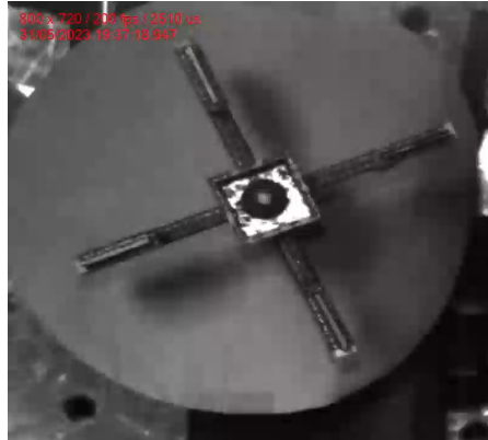
Video 3. “ Laser induced spinning ” of the simili Crookes mill target holder loaded with 1mm thick aluminum targets irradiated by a burst of 4 BIVOJ shots at 80J-10ns, 76GW/cm 2 : http://dx.doi.org/doi.number.goes.here
