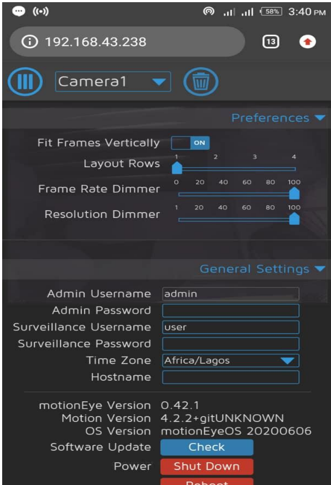
Figure 8. Open source configuration for motion activated camera.
