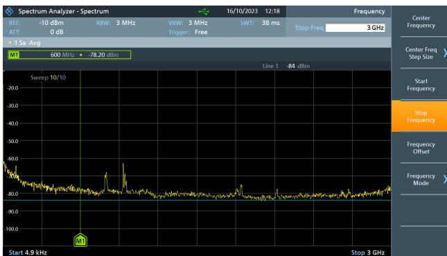
Fig. 6. Power density spectrum of the NC302BL
