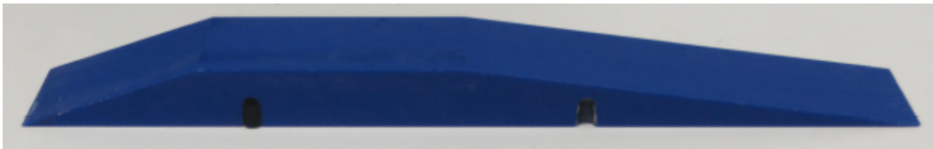
Figure 3. Image of an obstacle with the reference geometry ACRI 2010 [28]. The length of the obstacle is L = 32.2 \text{ cm} and the maximum height is b_{\max} = 2.1 \text{ cm} .
