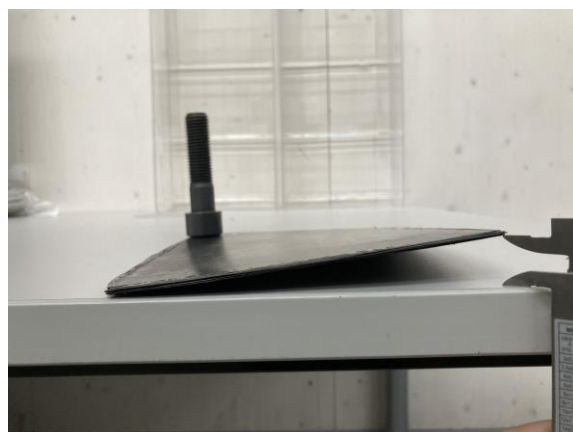
Figure 5. Warpage measurement of a consolidated plate.
