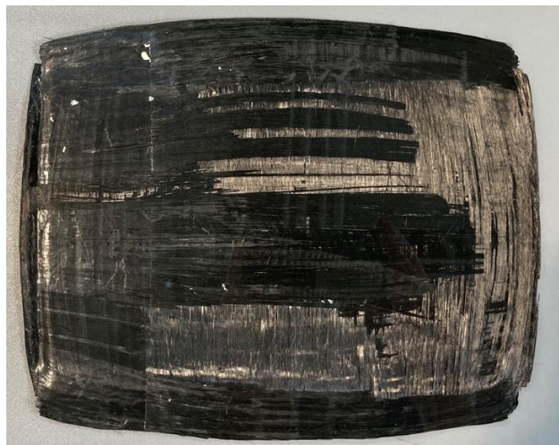
Figure 8. A split-open sample produced at 300 °C heating press temperature and 5 bar heating press pressure. The fibers at the sides deviate from their original orientation.
