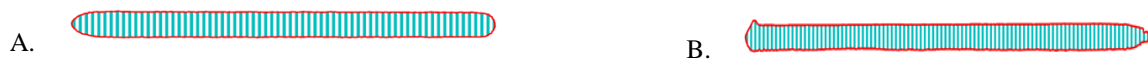
Fig. 8. A. – Width and B. – Height automatically computed along the printed filament with image processing
