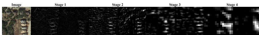
Fig. 1. Some examples of features extracted at different stages of the Gabor Encoder. The deeper the stage goes, the lower the resolution is. Notice that regions with buildings are clearly highlighted at each resolution, while other regions (in spite of being textured but without regularity) are suppressed in the feature maps.
