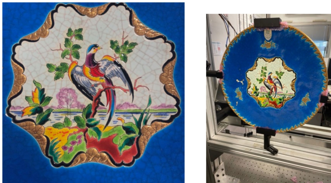
Figure 1. Picture of the plate (a) center and (b) global view of the sample (diameter of the plate: 45 cm).
