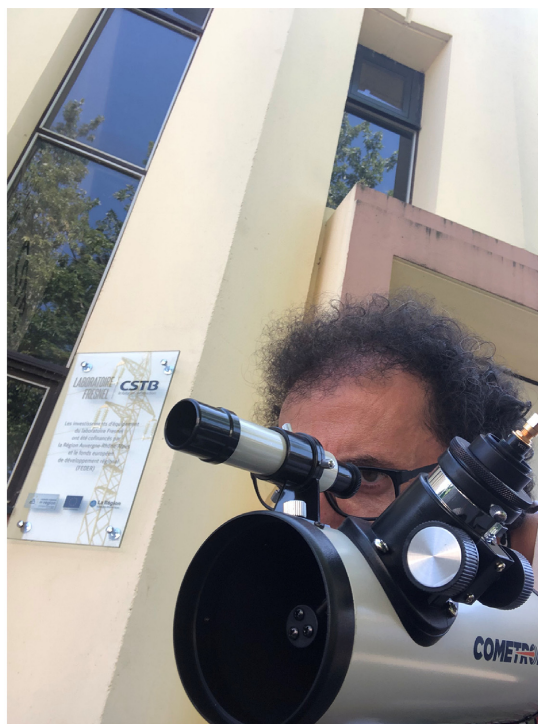
Figure 5 Photograph of the remote sensing telescope designed to measure TLM on site
