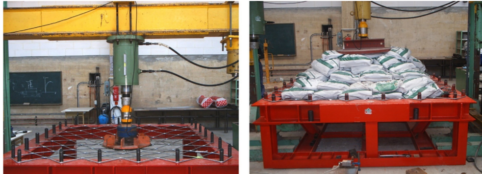
Fig. 5 Concentrated and distributed load punch tests on a cable net. Pictures from Castro-Fresno et al (2008) .
