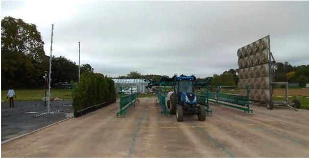
**Fig. 12.** Complete view of the drift test platform during the trials carried out in the presence of the hedge.
