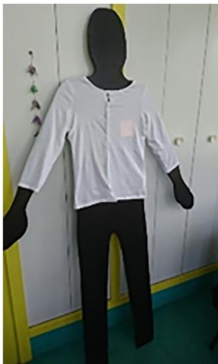
**Fig. 8.** Manikin used to measure drift deposition on bystanders.
