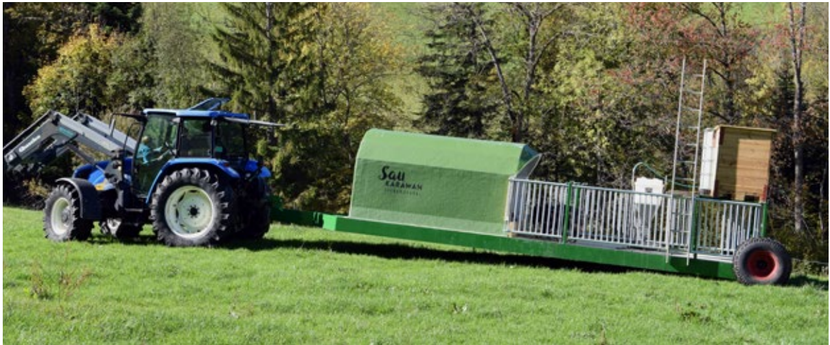
The "pig caravan" can easily be moved with a tractor, thanks to its two wheels and coupling device.
