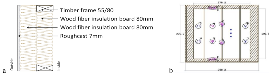
Fig. 1. (a) Wall structure (b) Measurement points in the walls mounted on PASSYS test cell,.
