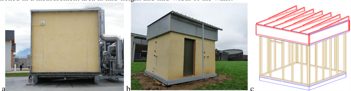
Fig. 2. (a) Photography of one of INES cells, (b) Photography of LERMAB test cell, (c) LERMAB test cell structure.
