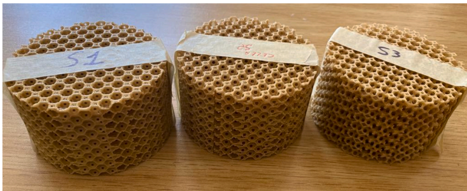
Fig. 9. An image of 3D printed membrane structures for experimental tests.
