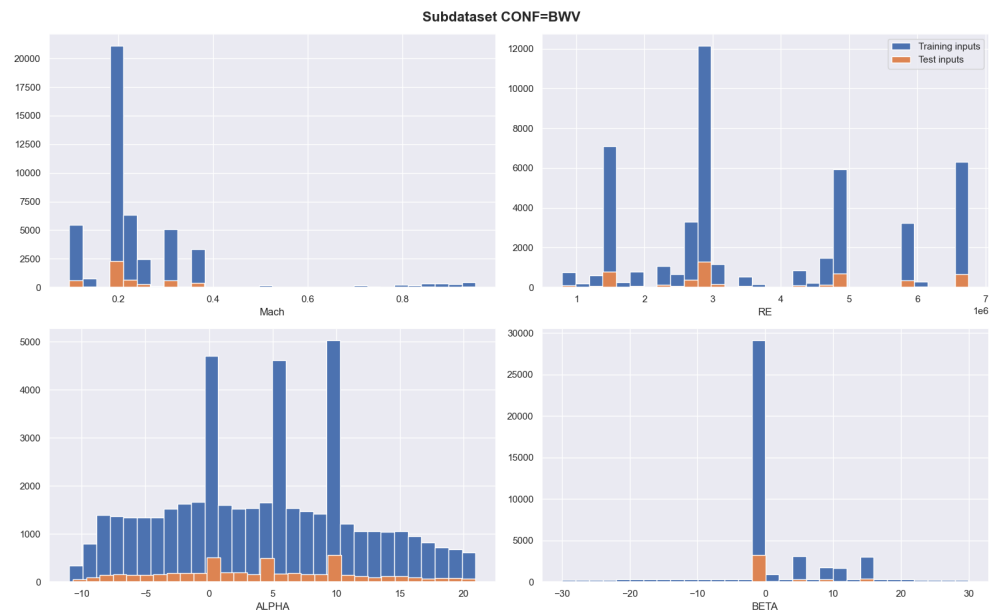
Figure 7. Histograms of the four input variables ( Mach , Re , \alpha , \beta ): training points (47,004 points in blue) and test points (5223 points in orange).
