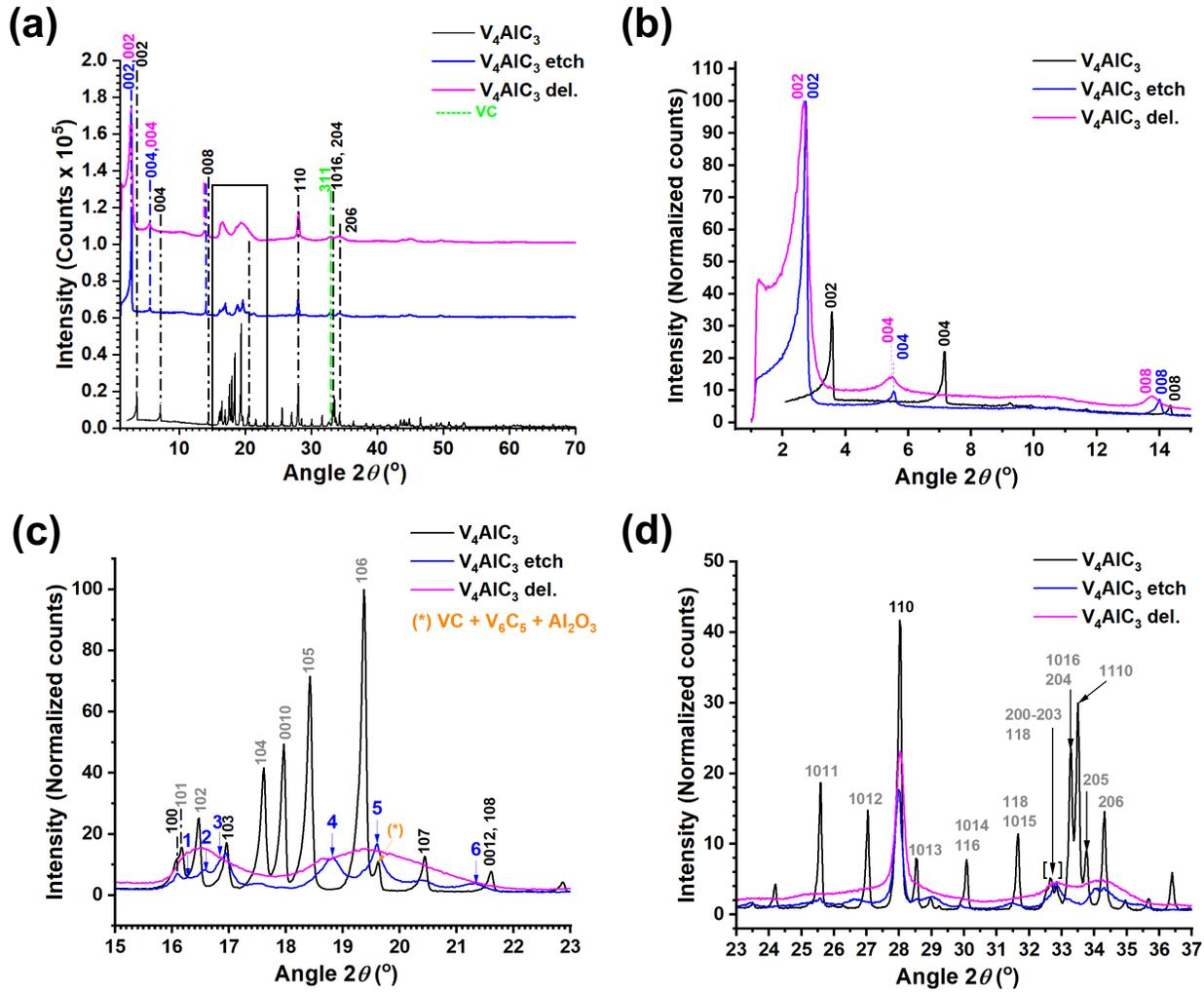
Figure 4: XRD patterns of  $V_4AlC_3$  and corresponding etched and delaminated samples. (a) Full  $2\theta$  range patterns, (b-d) patterns in reduced  $2\theta$  regions - for (c) the  $2\theta$  marked with a square in (a). The labels indicate hkl reflections corresponding to each sample (color set on the legend). In (b) hkl reflections present in  $V_4AlC_3$  but not on etched/delaminated material are marked (gray color).
