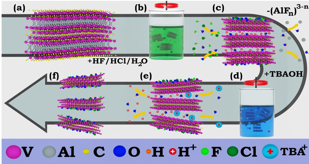
Figure 1: Synthesis procedure: (a)  $V_4AlC_3$  and an acid mix are combined in an (b) etching reaction to yield (c) multilayer  $V_{4-x}Al_{1-y}C_3T_z$  and subproducts, (d) the multilayer material is then combined with TBAOH in a delamination step where (d)  $H^+$  are exchanged with  $TBA^+$  ions to deliver (e)  $V_{4-x}C_3T_z$  delaminated flakes.
