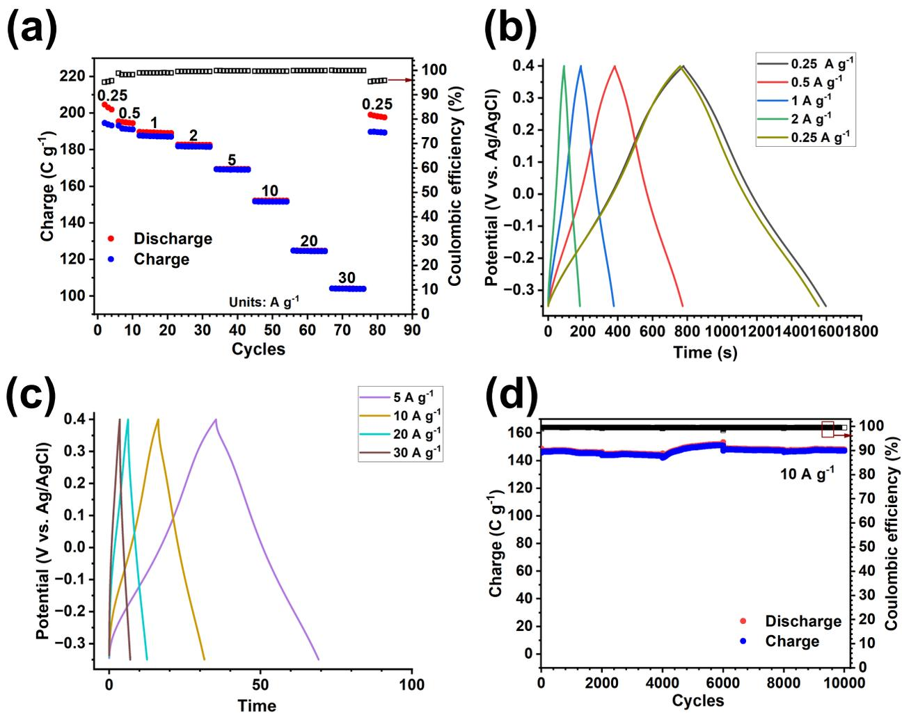
Figure 6: GCPL tests of  $V_4C_3T_z$  film electrodes performed in a half-cell set up using Ag/AgCl as reference electrode and 3 M  $H_2SO_4$  electrolyte. (a) Charge storage vs. cycle number curves obtained from GCPL tests at various current rates, (b-c) corresponding GCPL curves (second cycle), (d) Charge storage vs. cycle number curves for a cycling stability test performed at 10  $A g^{-1}$ .
