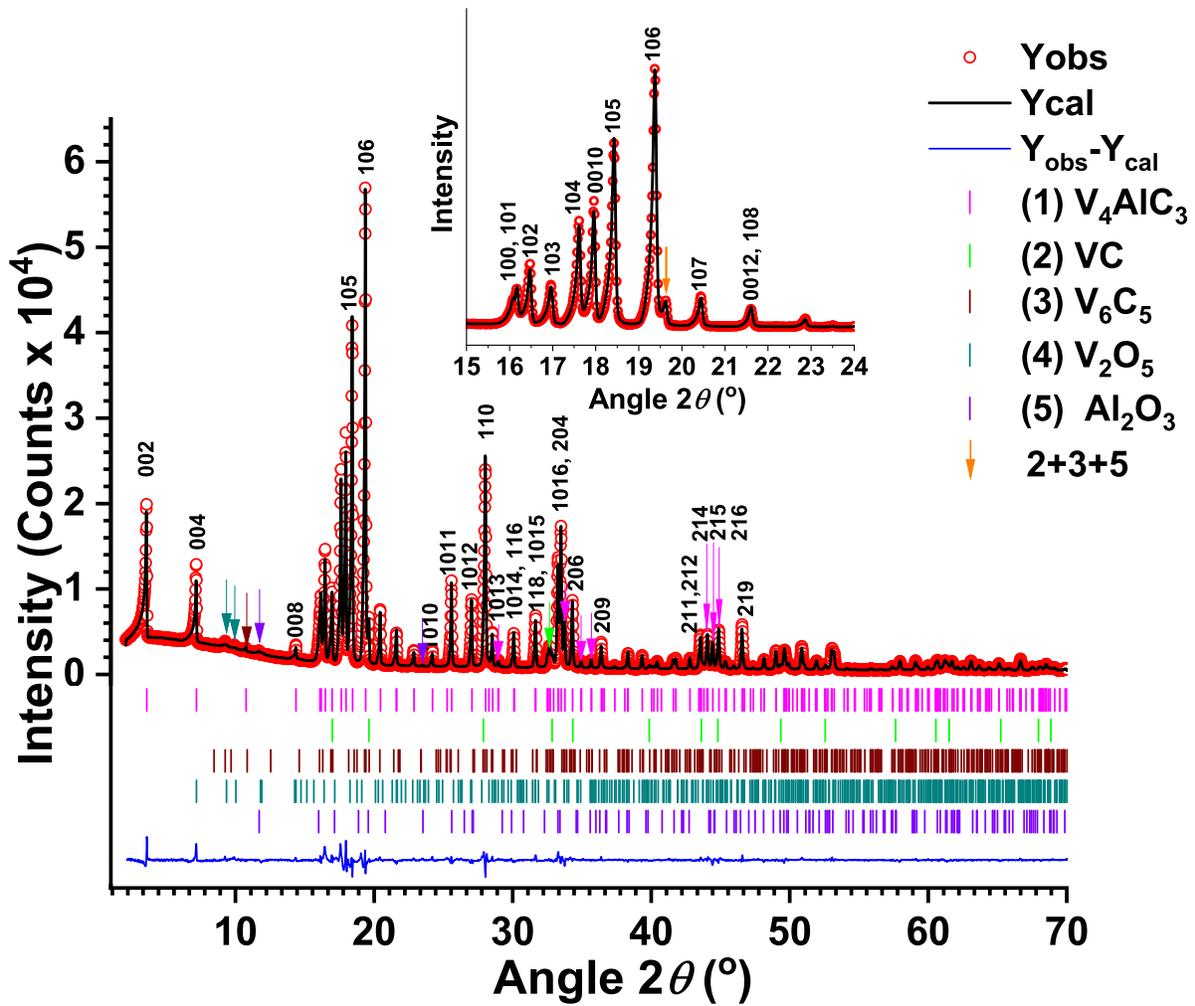
Figure 3: XRD pattern of  $V_4AlC_3$  and calculated model from Rietveld refinement.
