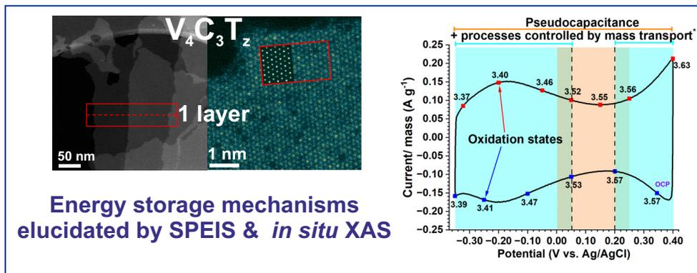
**Description:** Monolayer  $V_4C_3T_z$ , its atomic structure and elucidated charge storage processes at specific potential regions. \*The contribution of processes involving mass transport control are minor.
