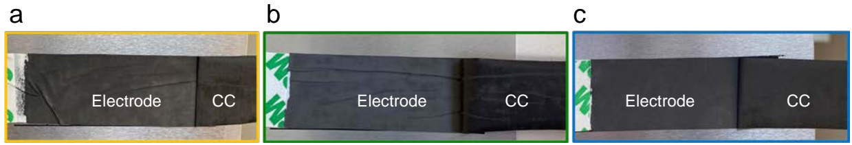
Figure S8. Electrode and current collector (CC) interface after peel tests. (a) 1-DSE, (b) 3-DSE and (c) 15-DSE.
