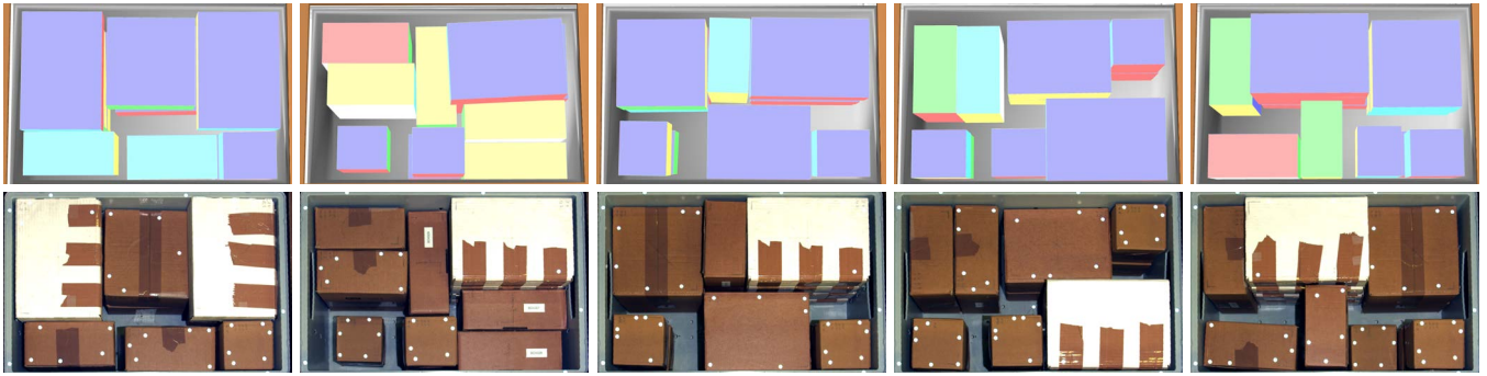
Fig. 7: Packing results as obtained from experiments (top row) and simulation (bottom row). Each column represents a different sequence.
