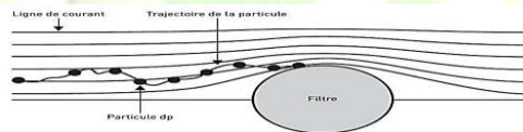
Figure 2: Schematic of the Brownian diffusion collection mechanism (Bémer et al. , 2006, and Colin, 2013).
