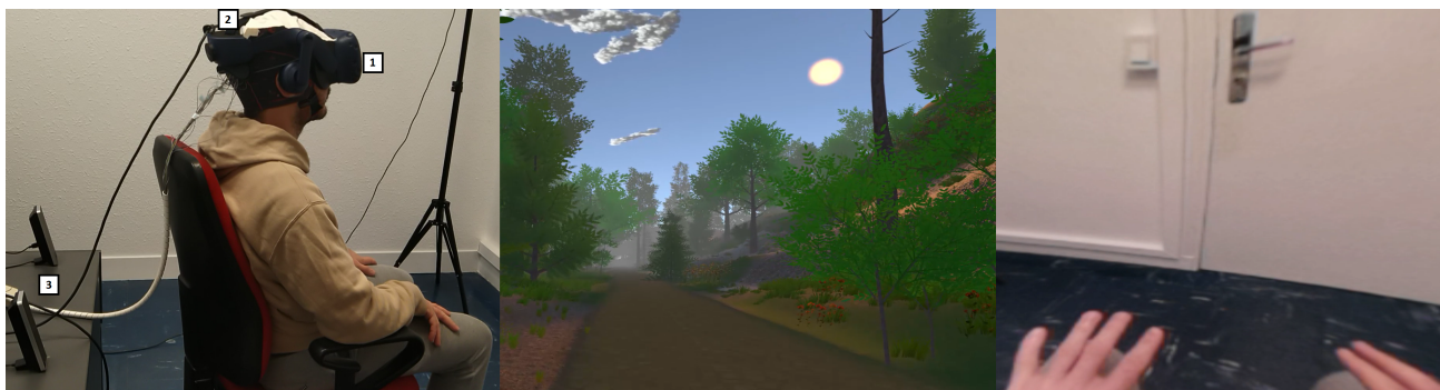
Figure 1: Experimental setup. Left: The user, equipped with the VR headset (1) and EEG cap (2), and the loudspeakers (3) producing oddball stimulus. Middle: Virtual environment developed to induce presence. Right: User’s view during a Break in Presence showing in real-time the real environment within the headset.
