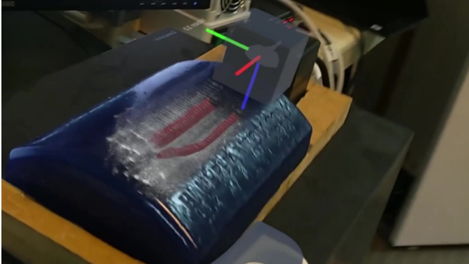
Fig. 6. 3-D volume reconstruction placed over the acquisitions' location, accurately representing the underlying medium.
