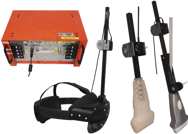
Fig. 2. Material used in the framework. ULA-OP [8] research platform (top left), 3-D tracked AR headset (bottom left), mock ultrasound probe (middle) and ultrasound probe (right)
