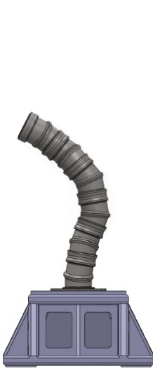
Fig. 2: Robot NB-R1 formed of six NB-modules
