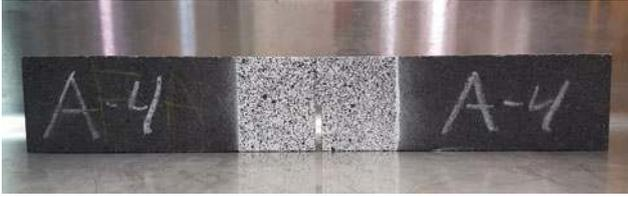
**Fig. 2** Typical carbon cathode sample used for stress intensity factor tests
