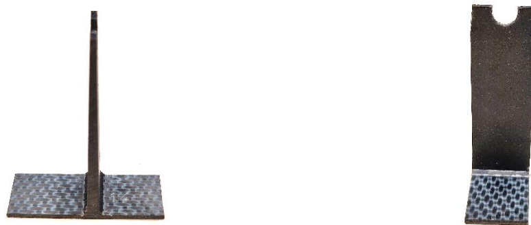
Figure 4. 20 mm-wide T joint used for testing, after recut
