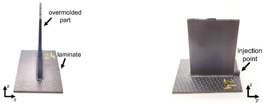
Figure 3. Original T joint structure as produced, before recut
