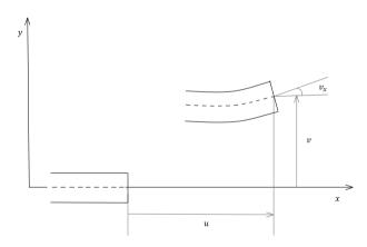
Fig. 3. Undeformed and deformed beam.
