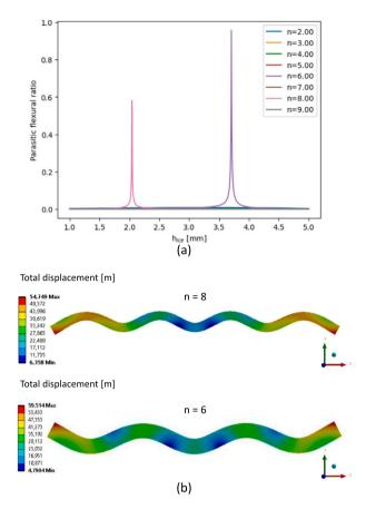
**Fig. 5.** (a) Analytical analysis of parasitic flexion using Rayleigh–Ritz approach. The peaks in parasitic flexion correspond to the superimposition of the flexural mode characterized by n antinodes, which leads to an increase in the parasitic flexural ratio. (b) FEM extensional modes for the first peak (n = 8) and the second peak (n = 6).
