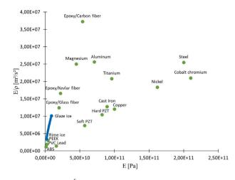
Fig. 6. Ratios  $\frac{E}{2}$  of different materials compared to those of ice.
