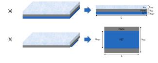
Fig. 8. Multilayered material geometry.
