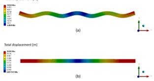
**Fig. 4.** 2D extensional mode for two different beams with 2.5 mm of ice accreted on top: (a) the beam is constituted by a titanium alloy, having an  $\frac{E}{\rho}$  ratio different from that of ice (b) the beam is constituted by a fictitious material having  $\frac{E}{\rho}$  equal to that of ice.
