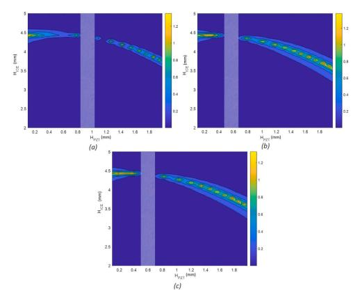
Fig. 9. Numerical calculation of the parasitic flexural ratios as a function of piezoelectric (PZT) transducer and ice thicknesses using (a) PIC181, (b) PIC151, (c) PIC255.
