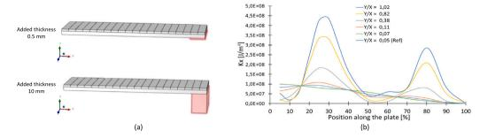
Fig. 2. Parasitic flexural ratio effect: (a) titanium plate with ice accumulated on top with a local mass added to generate parasitic flexion (b)  $K_{\chi}$  indicator as a function of the position along the plate.
