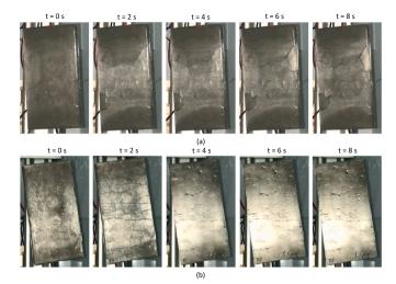
Fig. 14. 260Vpk extensional de-icing of a 3.5 mm thick ice layer: (a) Reference substrate (b) Partially multilayered substrate.
