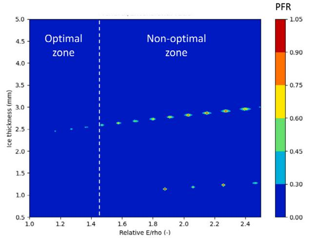
Fig. 7. Parasitic flexural ratio function of substrate material properties.
