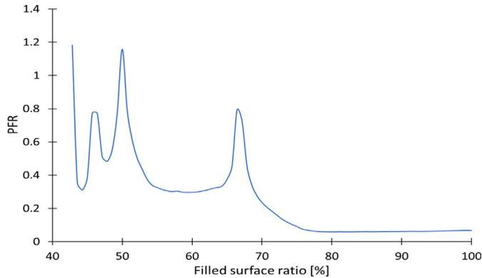
Fig. 10. Numerical calculation of the parasitic flexural ratio as a function of the PZT/titanium surface ratio.
