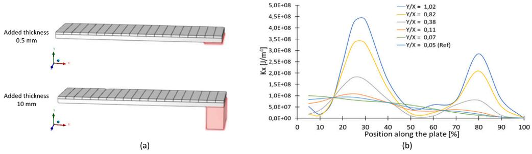
Fig. 2. Parasitic flexural ratio effect: (a) titanium plate with ice accumulated on top with a local mass added to generate parasitic flexion (b)  $K_x$  indicator as a function of the position along the plate.
