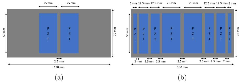
Fig. 11. Bottom view of the two titanium prototypes ( $130 \times 70 \times 1 \text{ mm}^3$ ): (a) Reference substrate (b) Partially multilayered substrate.
