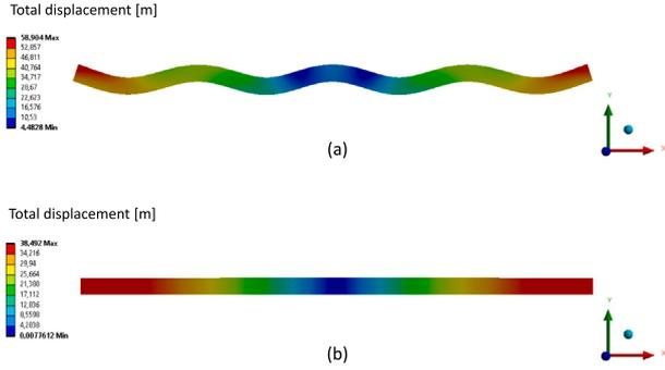
Fig. 4. 2D extensional mode for two different beams with 2.5 mm of ice accreted on top: (a) the beam is constituted by a titanium alloy, having an  $\frac{E}{\rho}$  ratio different from that of ice (b) the beam is constituted by a fictitious material having  $\frac{E}{\rho}$  equal to that of ice.
