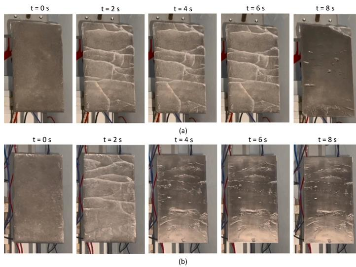
Fig. 16. 260Vpk extensional de-icing of a 4.5 mm thick ice layer: (a) Reference substrate (b) Partially multilayered substrate.
