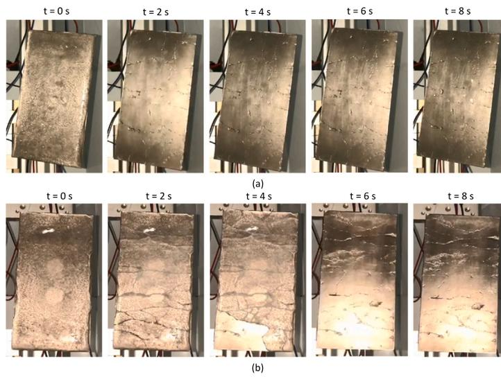
Fig. 15. 260Vpk extensional de-icing of a 4 mm thick ice layer: (a) Reference substrate (b) Partially multilayered substrate.
