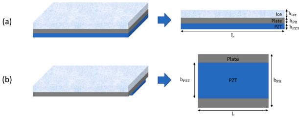
Fig. 8. Multilayered material geometry.
