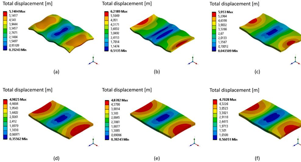
Fig. 13. Modal shapes of the extensional mode for the partially multilayered substrate with (a) 2 mm of ice (15.7 kHz, PFR = 0.57), (b) 2.5 mm of ice (15.5 kHz, PFR = 0.33), (c) 3 mm of ice (15.4 kHz, PFR = 0.34), (d) 3.5 mm of ice (15.3 kHz, PFR = 0.15), (e) 4 mm of ice and (15.2 kHz, PFR = 0.11), (f) 4.5 mm of ice (15.1 kHz, PFR = 0.15).
