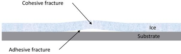
Fig. 1. Ice fracture mechanisms: cohesive and adhesive fractures.
