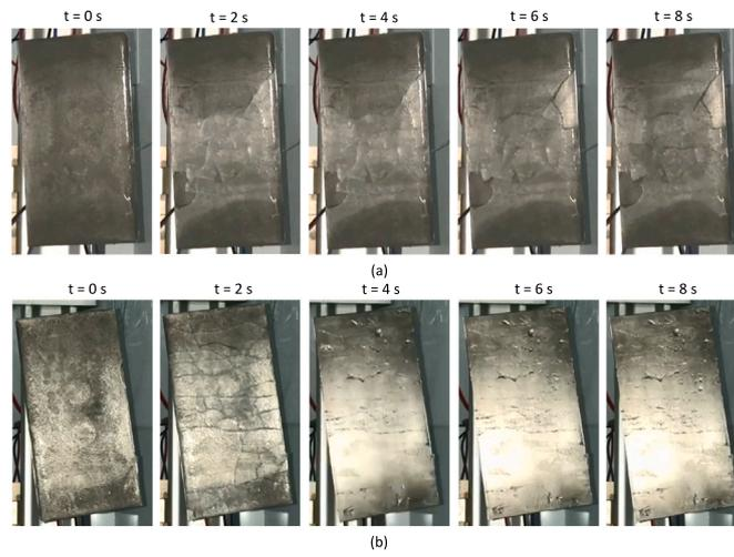
Fig. 14. 260Vpk extensional de-icing of a 3.5 mm thick ice layer: (a) Reference substrate (b) Partially multilayered substrate.
