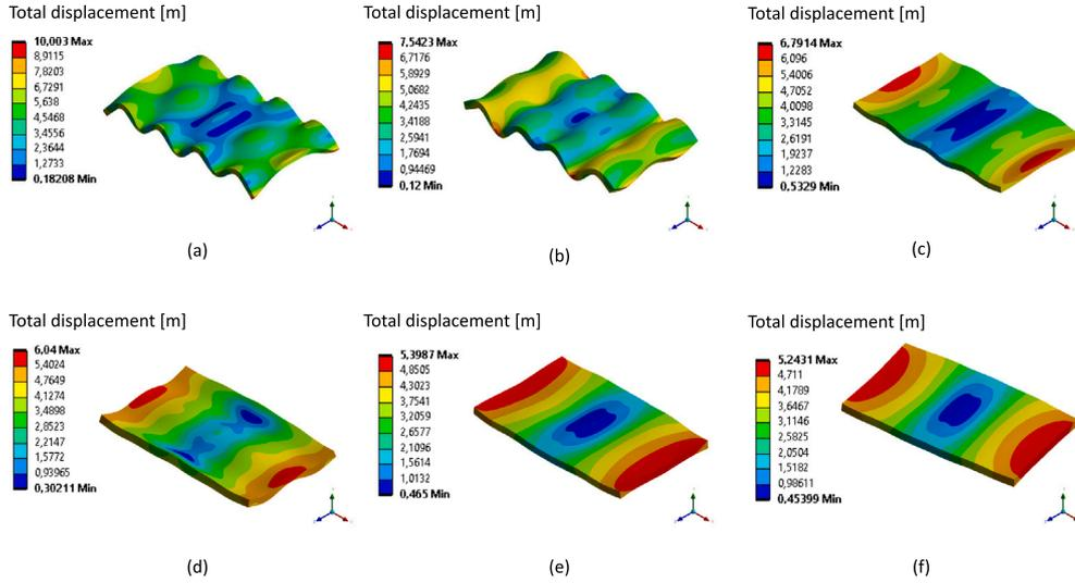
Fig. 12. Modal shapes of the extensional mode for the reference substrate with (a) 2 mm of ice (17.7 kHz, PFR = 1.26), (b) 2.5 mm of ice (17.6 kHz, PFR = 1.04), (c) 3 mm of ice (17 kHz, PFR = 0.3), (d) 3.5 mm of ice (16.9 kHz, PFR = 0.62), (e) 4 mm of ice and (16.6 kHz, PFR = 0.15), (f) 4.5 mm of ice (16.5 kHz, PFR = 0.13).
