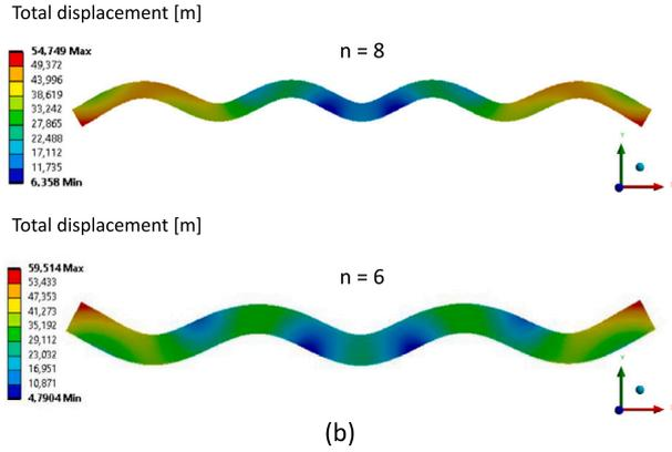
Fig. 5. (a) Analytical analysis of parasitic flexion using Rayleigh–Ritz approach. The peaks in parasitic flexion correspond to the superimposition of the flexural mode characterized by  $n$  antinodes, which leads to an increase in the parasitic flexural ratio. (b) FEM extensional modes for the first peak ( $n = 8$ ) and the second peak ( $n = 6$ ).
