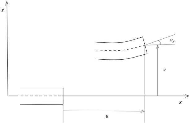
Fig. 3. Undeformed and deformed beam.
