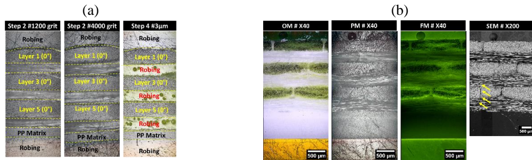
Figure 2. (a) Surface state evolution following during first polishing (step 2) and following mirror finishing (step 4). (b) Images of the same surface polished at 4000 grit following the first robing step and observed using OM, PLM, FM and SEM.
