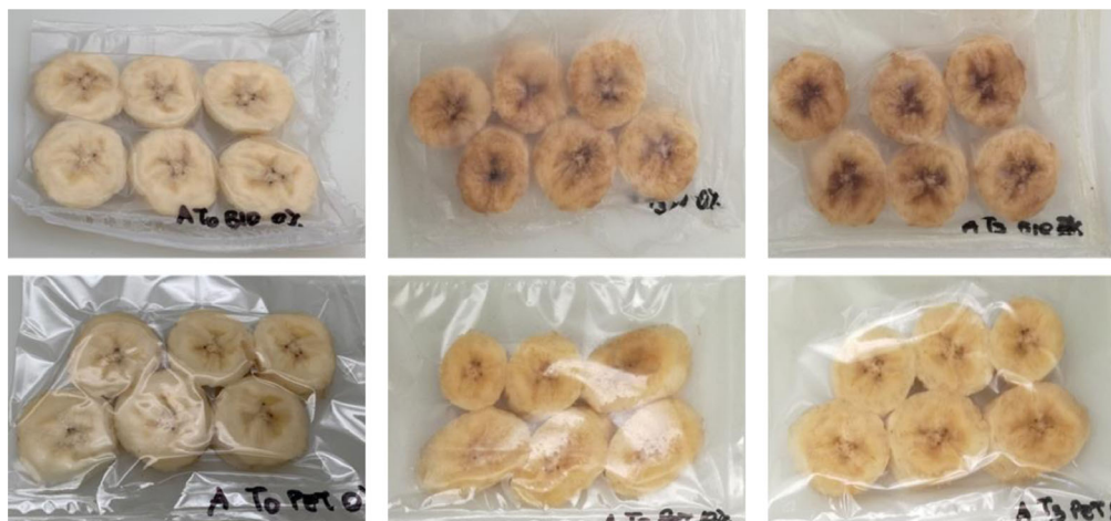
Figure 4. Pictures of banana slices. Top line: PLA/PBAT-based films; bottom: PET-based films. From left to right: slices at day 0; slices at day 3 in control condition; slices at day 3 in films coated with 5% active phase. PBAT, polybutylene adipate terephthalate; PET, polyethylene terephthalate; PLA, polylactic acid.
