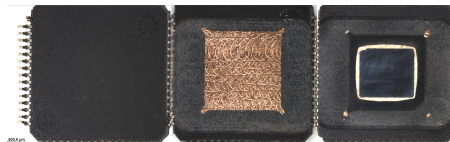
Fig. 10: Backside depackaging. Left: target before decapping. Center: resin removed. Right: copper layer removed, backside silicon exposed
