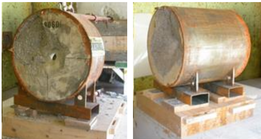
Figure 15. Post test images of the perforation concrete target (left, H = 300 mm) and the penetration concrete target (right, H = 800 mm).
