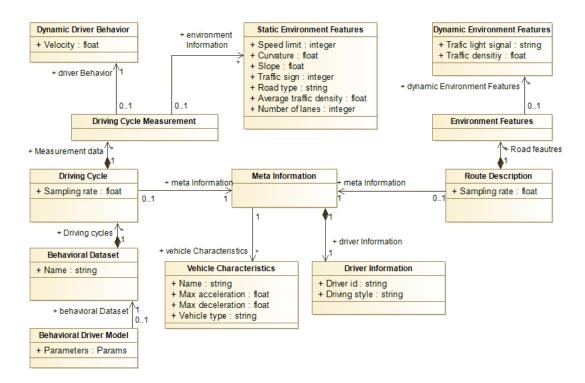
Figure 12: An excerpt of the AVL RDE data model
