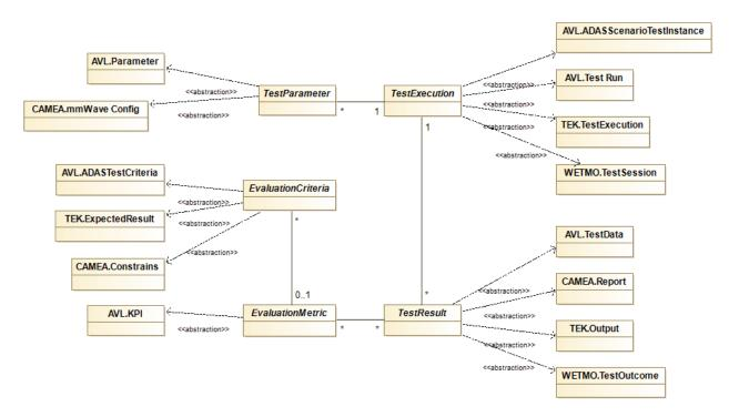
Figure 11: An excerpt of the Testing data model, its abstract elements, and the links to the case study related concrete elements.
