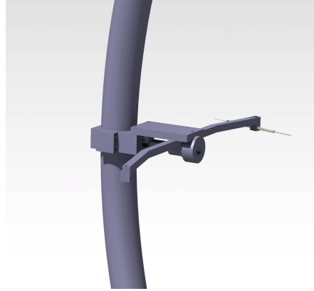
Figure 3. CAD image of the LP4 Langmuir probe setup. The LP is not aligned with the rotating arm.
