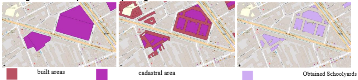
Figure 1. From left to right: after identifying the school in the land register, then the built areas, we isolate the schoolyard by subtracting the second from the first.
