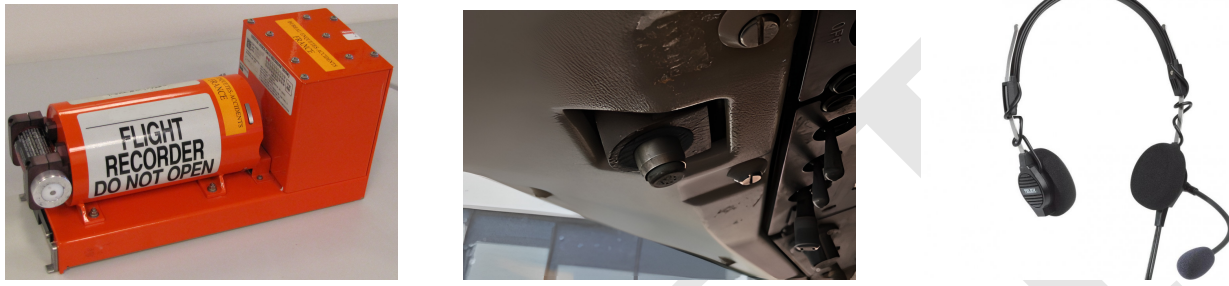
Fig. 3. Examples of a CVR system (left), a CAM (center), and a pilot headset (right).
