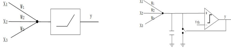
Fig. 3. Spiking neuron (right) and non-spiking neuron (left) circuit primitives
