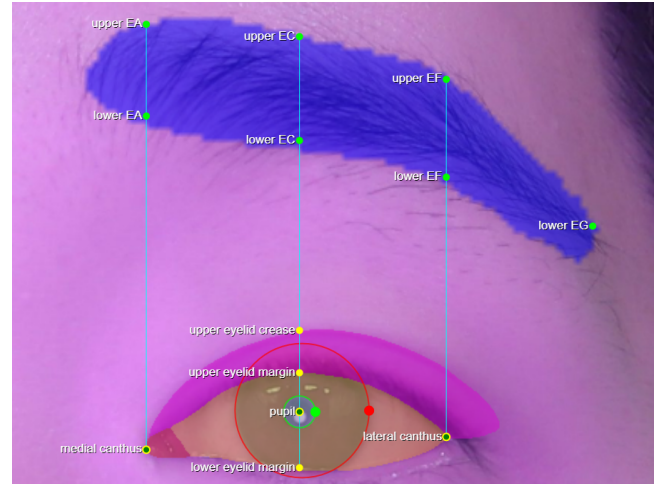
Figure 4: Detected and aligned points of eyebrow area (upper and lower). Points are named in order of A,C,F and G.
