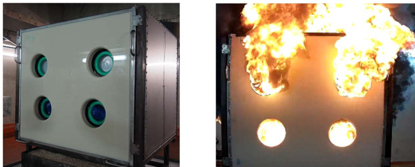
Fig. 13 Glove box fire tests with the kyowaglas surrogate panels. View from the front side of the glove box before the fire (a). View from the rear side of the glove box during the fire (b).
