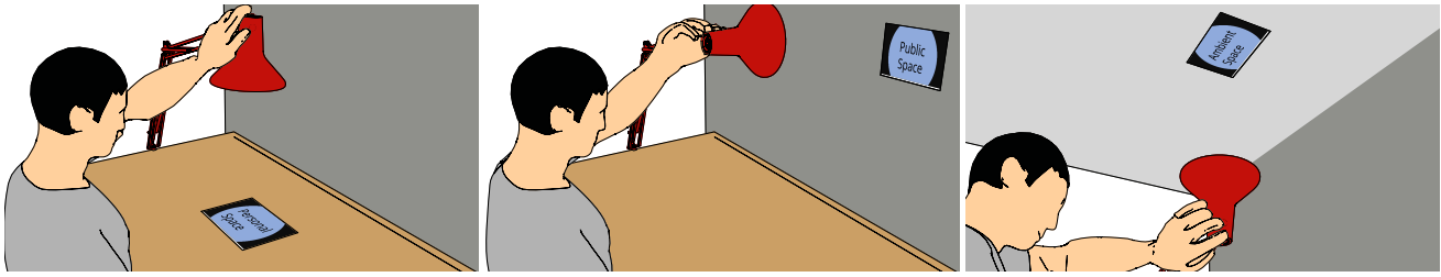
Figure 4: The content in the window adapts to the change of surface when users manipulate LuxAR.
